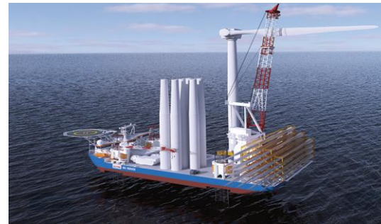
해상풍력설치선 (Wind Turbine Installation Vessel)
